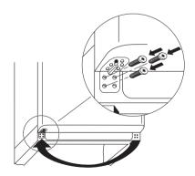
**18.** Open the freezer compartment door and fit the plinth.
